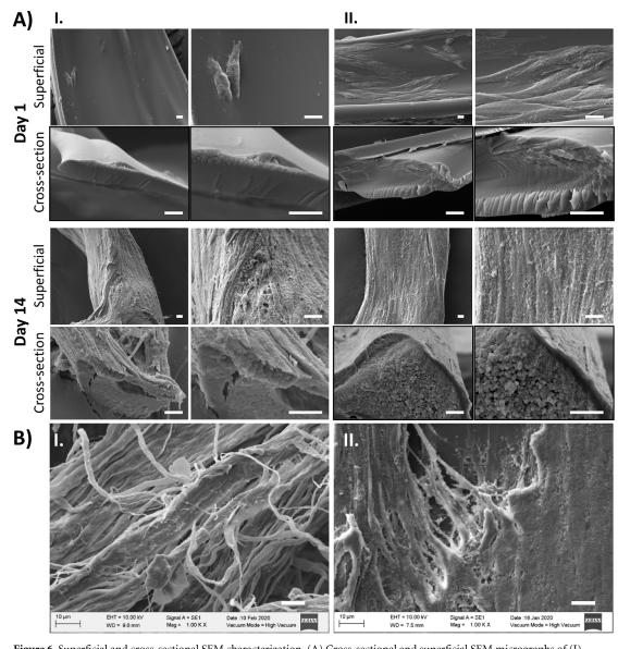
**Figure 6.** Superficial and cross-sectional SEM characterization. (A) Cross-sectional and superficial SEM micrographs of (I) GelMA and (II) GelMA-TuMV fibers. Scale bars: 10  $\mu$ m. (B) Comparison between real muscle-tissue and artificial muscle-like constructs. SEM micrographs from (I) native mammal muscle tissue and (II) lab-made fiber (GelMA-TuMV) after 14 d of culture. Scale bar 10  $\mu$ m.
