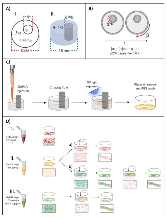
**Figure 1.** Experimental strategy. (A) MiniJB device (I) dimensionless parameters and (II) actual dimensions, (B) representation of one cycle of the process, (C) schematic diagrams of fiber fabrication process and (D) different types of fibers fabricated: (I) GelMA with fluorescent particles (FP), (II) pristine GelMA (a) cell-seeded or (b) with a superficial TuMV coating followed by a cell-seeding process, and (III) GelMA with embedded TuMV and subsequent cell-seeding.
